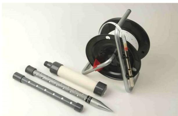
**PIEZOMETER** Measure Pore
